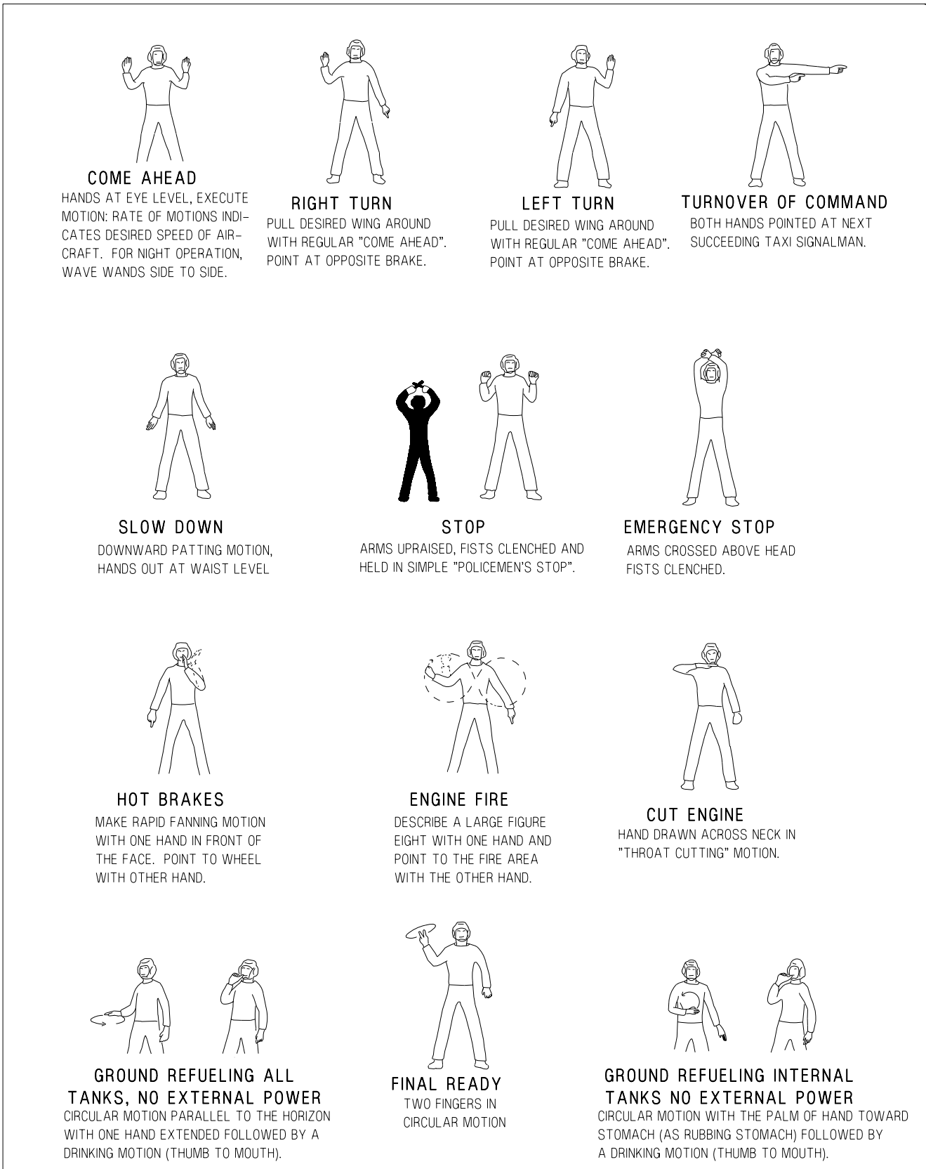
Figure 27-1. Deck Ground Handling Signals (Sheet 3 of 4)
